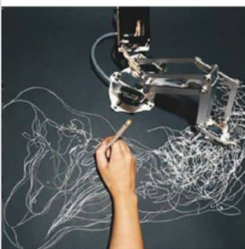
Drawing Operations Unit: Generation 1 (DOUG 1) was the first of Chung’s collaborative robots.
