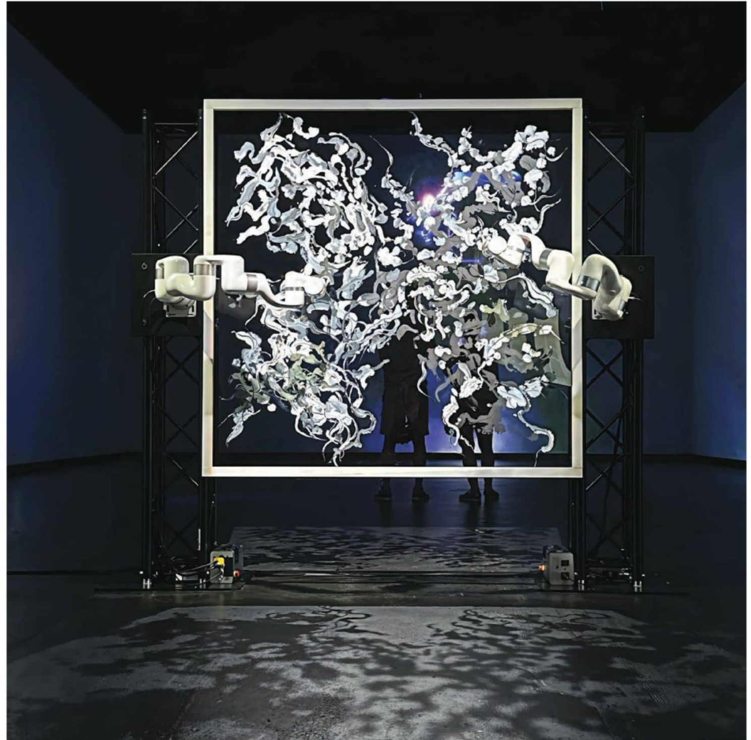
Spectral , a performative art installation presented in January, featured robotic arms whose drawing motions were guided by real-time input from an EEG worn by the artist.
